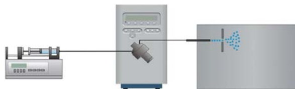
Fig.4. ROXY™ EC System including ReactorCell™ and dual syringe infusion pump.
