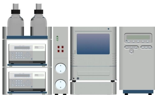
Fig. 1. ALEXYS Aminoglycosides analyzer for Spectinomycin
