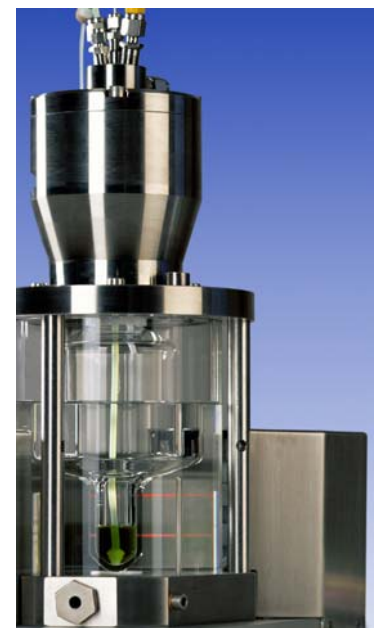
Laser controlled vacuum chamber
