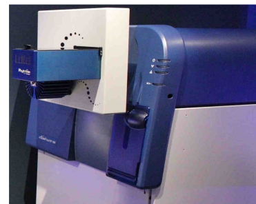
Figure 2 LDTD- AB Sciex TripleTOF™ 5600
