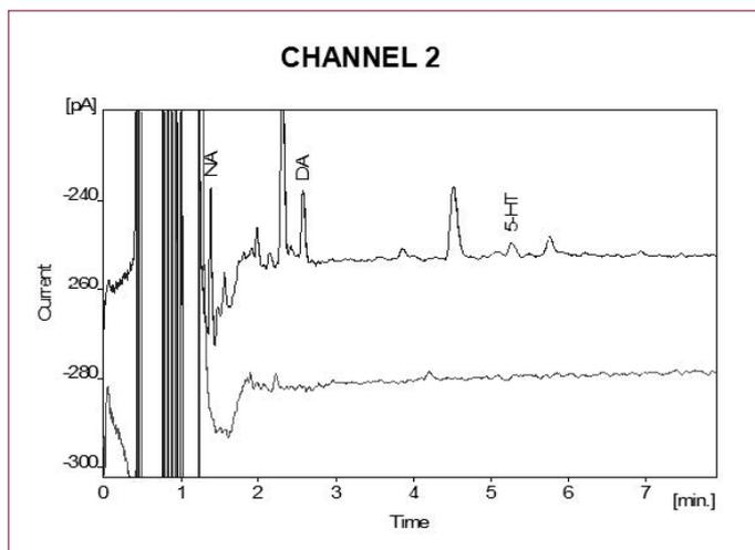
**Figure 5:** Analysis from a single injection of basal level rat Prefrontal Cortex (PFC) microdialysate. In both chromatograms the bottom trace is an injection of blank (Ringer solution). Samples kindly provided by Mrs. Gerdien Korte-Bouws, Department of Psychopharmacology, University of Utrecht, The Netherlands.
